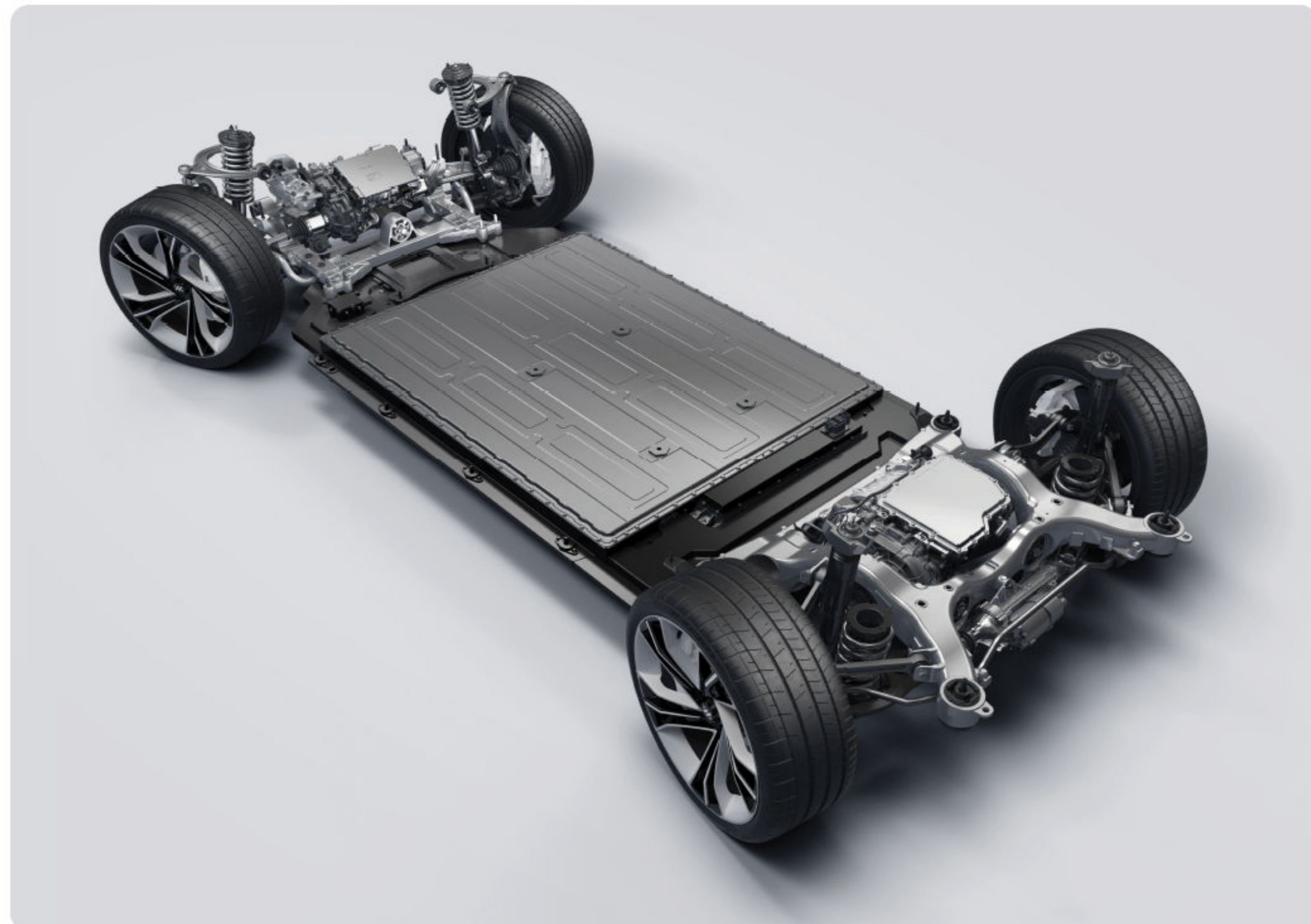
AKC (Four-Wheel steering system) CDC (Intelligent Electronically Controlled Suspension)
